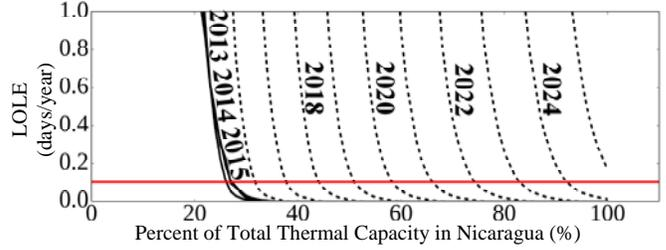
FIGURE III: NICARAGUA LOLE WITH REGIONAL CAPACITY (300 MW CONSTRAINT) AND REDUCED THERMAL CAPACITY
