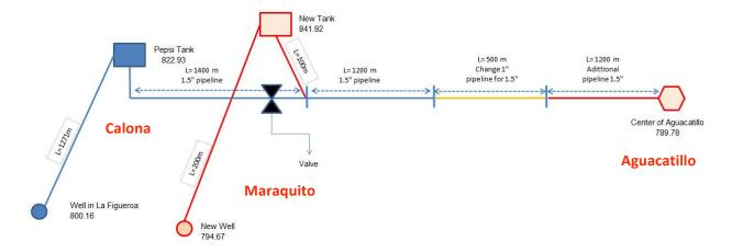
Figure 5. Future Distribution System. Calona will be split from the system by a valve and Maraquito and Aguacatillo will be serviced by the new system.<sup>5</sup>
