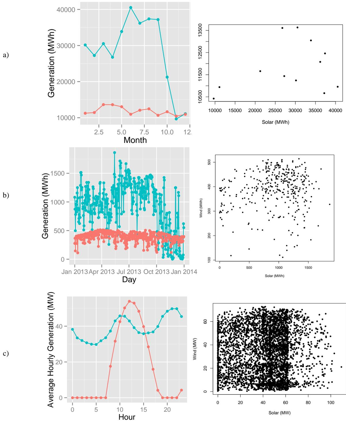
Fig 5. Monthly aggregate solar output (seven 15 MW central PV plants) and wind output: a) monthly,  $p_{X,Y}$  hourly=0.24, b) daily  $p_{X,Y}$  daily=0.18, and c) hourly  $p_{X,Y}$  monthly=0.42)
