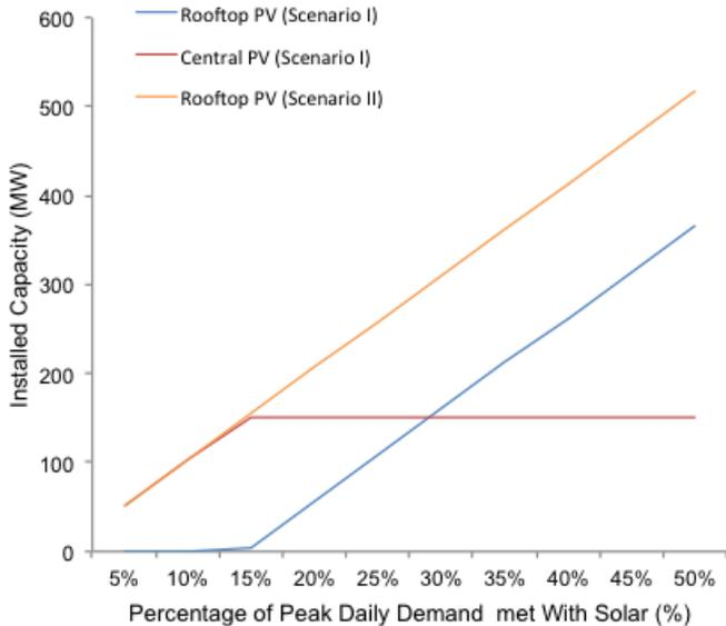
Fig. 4. Amount of rooftop and central PV installed capacity required to meet different levels of peak daily demand under two different cost scenarios (low and high central PV costs)
